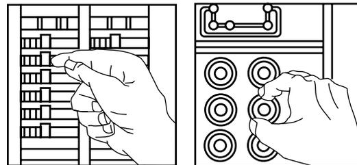
Next, plug in and turn ON the lamp or radio at the receptacle's other outlet to make sure the power is OFF at both outlets. If the power is not OFF, stop work and call an electrician to complete the installation.
