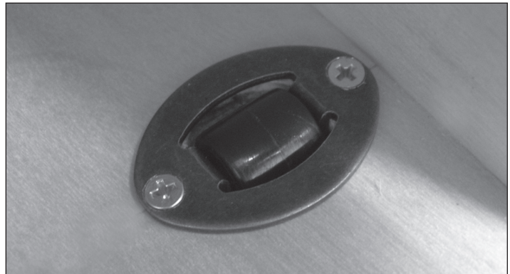
Figure 8 - Lubricate rollers with silicone spray
