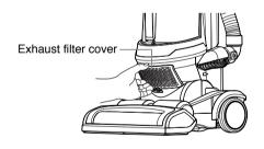
2. Lift out the filter by pressing the hook.
