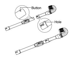
2. Attach the opposite side of the hose onto the main body.
