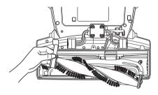
4. Hook the new belt over drive pulley of agitator motor.
