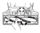
3. Unhook the old belt from the drive pulley. Make sure no pieces of the broken belt are trapped in the agitator or drive pulley area.
