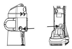
4. Check the hose where it connects body to head by turning the connector on the bottom of the body.
