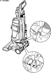
Release the hose assembly from the vacuum cleaner. Separate the hose and wand by pressing the button on the top of wand and check the hose and wand for clogs.
