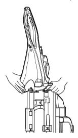
Note: Cord rewind button is in the up position when inserting into the main body. It is recommended to leave the tape on the button until the body and handle are assembled
