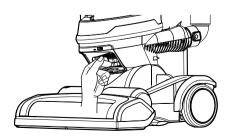
3. Wash the filter cleanly in flowing water.
