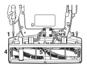
4. Carefully remove any accumulated string, hair, etc. from the agitator and the agitator area. To reinstall the cover.
