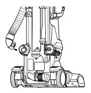
3. Align the hose with the holder on the side of the vacuum and place the end of the wand onto the main body.
