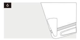
Replace the plastic hinge cover over the top hinge bracket.
