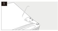
Using a flat blade screwdriver remove the plastic hinge cover from the top of the door.Be careful not to scratch the refrigerator surface.
