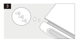
Using a thin-bladed tool,carefully pry up and remove the hole plugs on top of the door and the top of the opposite side of the cabinet. Insert plugs into the provided holes on opposite side of door and into the holes exposed by the removal of the top hinge bracket.
