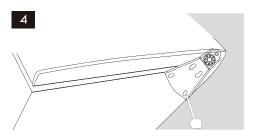
Using a slotted screwdriver, remove the two screws attaching the bottom hinge bracket to the refrigerator cabinet. Unscrew the foot from the other side of the cabinet. Avoid tilting the refrigerato more than 45 degrees when removing the bottom bracket and foot. Attach bracket and foot to the opposite side from where they were removed.
