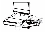
4) Loop the new belt over the motor drive shaft. Place the opposite end of the belt on the brush roll pulley.
