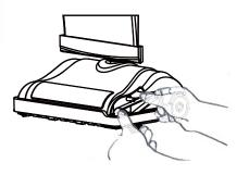
5) Rotate the brush roll several complete revolutions to ensure that no part of the belt is overhanging the end of the motor drive shaft.
