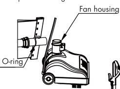
2.Remove the filter bag and check the inlet nozzle for any obstructions.
