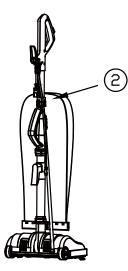
3.Press the cord into the cord clip, and ensuring the cord is fully rested in clip.
