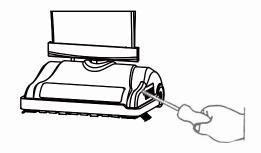
3) Remove the belt from the brush roll pulley and the motor drive shaft, clean the residue off the broken belt if needed.
