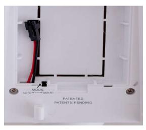
Fig. 3 SMART & AUTO Mode Factory default is SMART Mode
