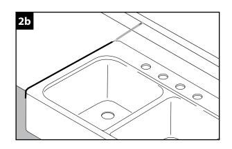
Using a jigsaw with a thin blade, cut inside the traced line from the front of the countertop to the front of the cabinet on both sides according to your measurements and figure 2c.
