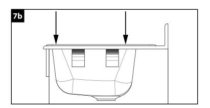
8. With sink sitting flush on counter top, apply downward pressure and shift sink side to side and front to back to make sure the clips "seat properly".
