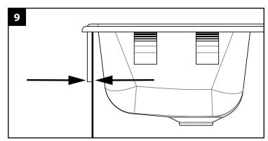
10. Apply a high grade of color-matched silicone. Apply the silicone around the sink, including the front apron.
