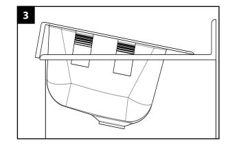
4. Remove the sink by pushing in on the side clips from underneath and pushing up gently on sink until free.
