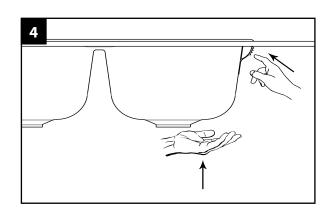
5. Peel back protective film around faucet, drain holes, and sink perimeter.
