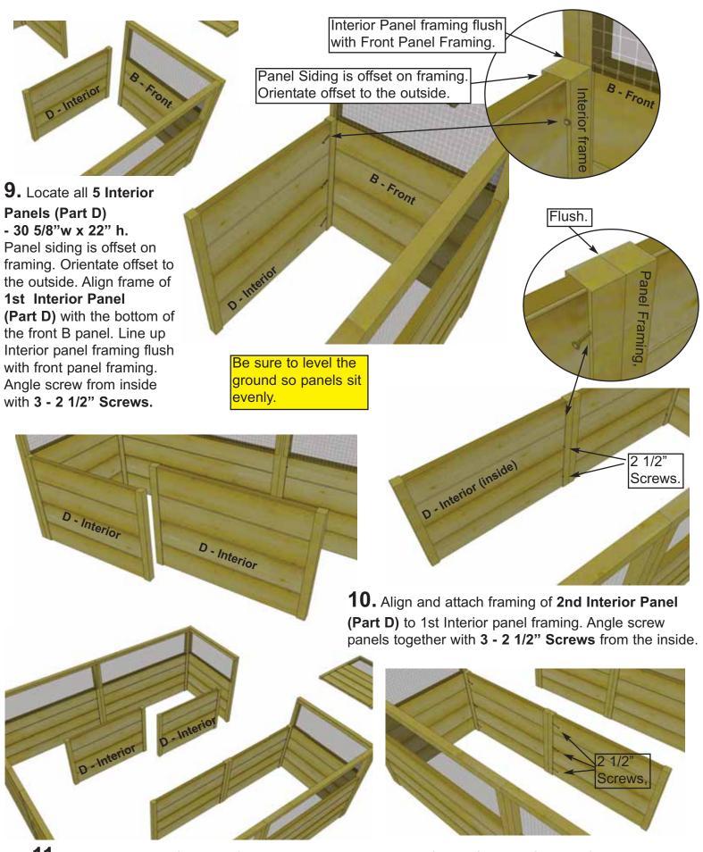
**11.** Align and attach framing of **3rd and 4th Interior Panels (Part D)** as per **Steps 9 & 10.** Angle screw panels together with **3 - 2 1/2**" **Screws** from the inside.
