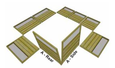
2. Starting in rear corner, position Rear and Side Panels (Part A) - 46" wide together so framing is flush at top and sides. When aligned, attach frames together at top with 1 - 2 1/2" Screw. Use Wood Clamp to hold frames together. Pre-drill rear frame first with 1/8" diameter bit to prevent wood from splitting.
