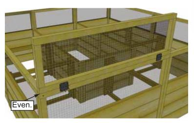
**23.** Line up side of back wall trellis/screen framing even with side wall framing. Attach hinges to rear wall framing with **3 - 3/4**" **Black Headed Screws** per hinge. Pre-drill shallow hole first to prevent wood from splitting.
