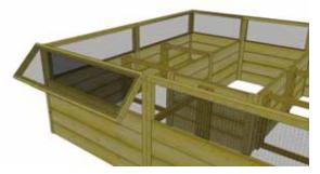
**24.** Complete attachments of both back wall trellis/screens to rear wall framing. Confirm screens can move up and down smoothly. Adjust if necessary.
