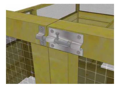
**26.** Attach **Silver Barrel Bolt** (male and female pieces) to side framing of trellis/screen. Use 6 - 3/4" **Silver screws**.
