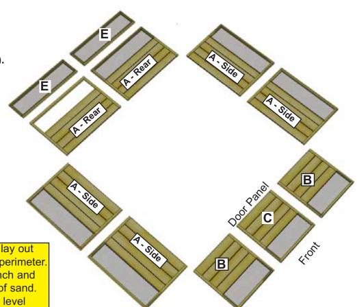
Before positioning panels, lay out footprint and level ground perimeter. If possible, dig a small trench and backfill with 1 or 2 inches of sand. Sand will make it easier to level panels.
