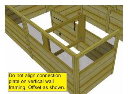
16. Lift and position completed short Bed Rib Frame and place between side and interior panel siding. Do not center on panel framing. Align with bottom of panels. Secure with 6 - 2" Screws per plate.
