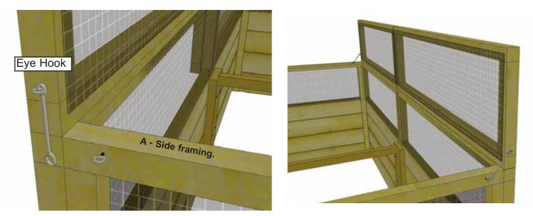
**25.** Lift trellis/screen into the up position. Screw male portion of **Eye Hook** into trellis/screen side framing and female piece into side framing of side wall. Do a dry run first to confirm correct position. Complete both sides.
