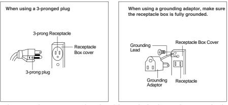
NOTE: THE CANADIAN ELECTRICAL CODE DOES NOT ALLOW THE USE OF THE GROUNDING ADAPTOR.
