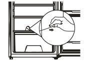
Please ensure the drain hole is checked and cleaned on a regular basis so water can exit the storage compartment.
