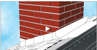
**9**Center the cricket flashing along the back of the chimney allowing the ends to extend 3 to 4 inches past. Notch out both ends even with their respective corner and bend tabs around to the sides. Nail in place.
