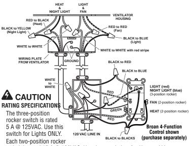
switch is rated 15 A @ 120VAC. Use these switches for Heat and Vent. The total load on this control must not exceed 20 A @ 120VAC.
