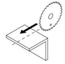
Corner Piece Feed blade diagonally through the work surface.
