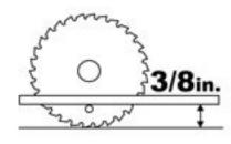
Thin Plate Feed blade down about 3/8" and start cut.
