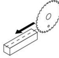
Flat Bar Iron Feed blade at a 90° angle to the work surface.
