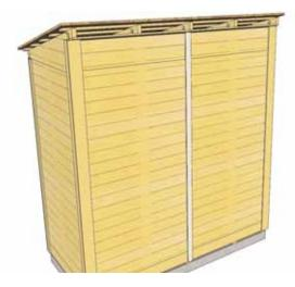
**56.** Attach **Middle Trim** - 1/2" x 2 1/2" x 88 3/4" where wall panels come together and leave a seam in the rear. Attach with 8 - 1 1/4" finishing nails aligning flush with bottom skirting.
