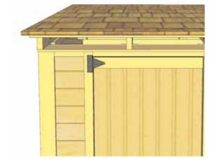
**60.** Make sure Door Panel is aligned evenly at top and edge. When aligned correctly, attach top and middle hinge to narrow trim with hinge hardware provided.
