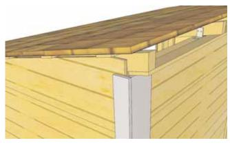
**55.** To completely trim out rear corners, locate **Rear Trim** -1/2" x 2 1/2" x 88 3/4" and a **Rear Corner Trim** - 1/2" x 4 1/2" x 88 3/4". Align and attach as per **Step 54**.
