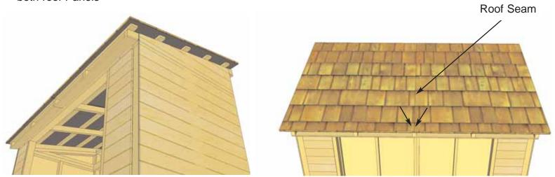
**39.** With Roof Panel aligned, screw panels down to center rafter with 2 - 2.5" screws in the bottom row of shingles. (1 screw per panel)
