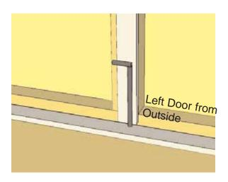
**70.** The Interior Cane Bolt will be attached to Vertical Door Flange. To position Cane Bolt correctly, attach to flange first, close doors and mark hole to house Cane Bolt Rod. Open doors and drill hole where previously marked with 9/16" bit. Use hardware and instructions provided in Cane Bolt kit to complete installation.
