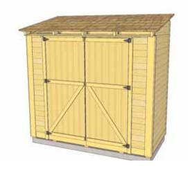
**61.** Place second Door into position and attach as per **Step 59**. Make sure Doors can open and shut correctly prior to completely securing hinge screws.
