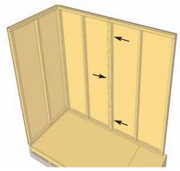
**13.** With the corner wall attachment complete, position the second rear wall panel in place so bottom 2x3 wall framing is sitting flush with outside floor joists and plywood floor. Wall siding should overhang floor by approximately 1/2". When positioned correctly, attach both wall panel studs together as per **Step 12** with 3 - 2 1/2" screws.
