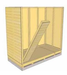
**15.** Secure side wall panel to rear wall panel as per **Step 12**. Next, locate **Narrow Wall Panels** and position in front corner.
