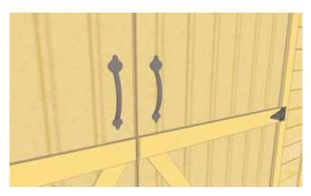
**71.** Attach **Door Handles.** Handles are positioned on top section of each door and mounted with 3/4" Black Screws.
