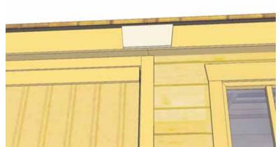
**73.** Attach **Facia/ Detail Plates** to cover seam where Front Facia pieces come together. Secure 4 - 1 1/4" finishing nails .
