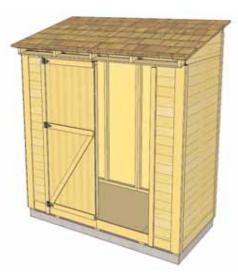
**58.** With Hinges attached on to door panel, position in doorway opening.
