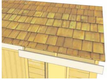
**63.** With Side Angle Cut Facia correctly aligned, attach Front Facia to rafter ends with 6 - 1 1/4" finishing nails per piece. Attach Side Angle Cut Facia to batten ends with 4 - 1 1/4" nails. Attach next piece of Front Facia. Align Facia in corner as per **Step 62**. **Note**, with Front Facia correctly aligned, a small gap may occur where they meet. This will be covered by Facia Detail Plate in **Step 73**.
