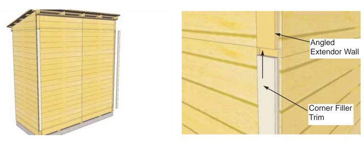
**50.** Position and attach Corner Filler Trims in the rear as per **Step 49.**
