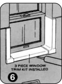
4. Apply adhesive to underside of sill. Cushion-seal foam strip is factory applied and provides a good seal for uneven edges. Be sure to center sill panel 3/4" away from each side wall. Vertical jamb panel will cover the gap. After positioning, follow "adhesive venting instructions" then final fit by pressing firmly into place.
