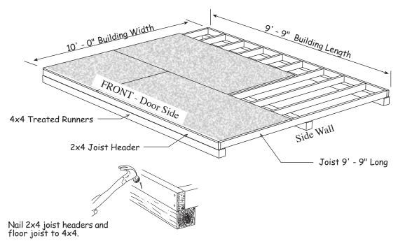
It is important that the floor be level and square. Before nailing the flooring, measure the floor diagonally (corner to corner). Then measure the opposite corners. These measurements will be the same if the floor is square.
