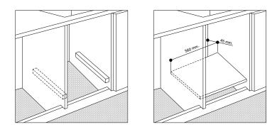
The panels of the adjacent cabinets must be made of heat-resistant material .In particular ,cabinets with a veneer exterior must be assembled with glues which can withstand temperatures of up to 100 .
