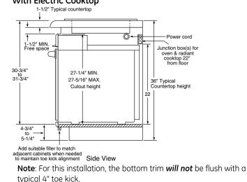
Note: Cabinets installed adjacent to wall ovens must have an adhesion spec of at least a 194°F temperature rating.
