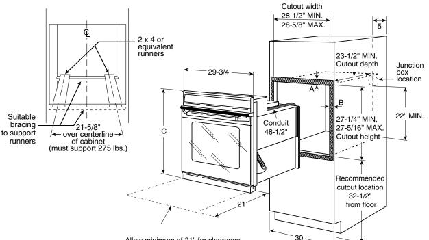
Allow minimum of 21" for clearance to adjacent corners, drawers, walls, or etc.
