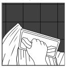
Fill joints completely. Remove excess grout with a float or squeegee as you go along.
