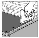
Fasten to the plywood with 1-1/4" DUROCK Brand Wood Screws or 1-1/2" hot-dipped galvanized roofing nails, spaced 8" o.c. in both directions and around edges. Leave a 1/8" gap between panels.
