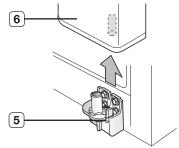
**4.** Remove the lower hinge 7 from the bracket 8 by gently lifting the lower hinge upwards.
