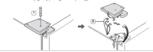
2. Remove hinge screws 4 and the ground screw 5 by turning counter-clockwise, and take off the upper hinge 6. Be careful that the door does not fall on you as you are removing it
