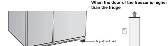
In the case of the process to correct the imbalance is the same. Open the doors and adjust them, one at a time, as follows:
