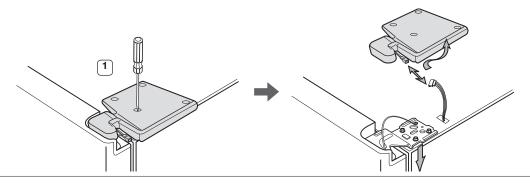
2. Remove hinge screws 2 and the ground screw 3 by turning counter-clockwise, and take off the upper hinge 4. Be careful that the door does not fall on you as you are removing it.
