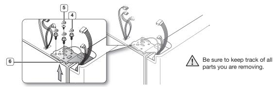
3. Next, remove the door from the lower hinge 7 by carefully lifting the door straight up 8.
