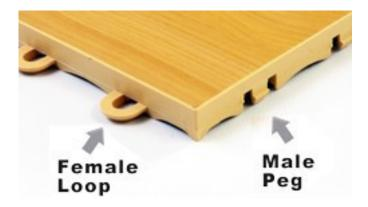
**Step 2** Start by laying your first panel in any corner (male edges required) or garage opening (female edges required) roughly 1" from the wall. The loops should be pointed in the direction you want to add panels:
