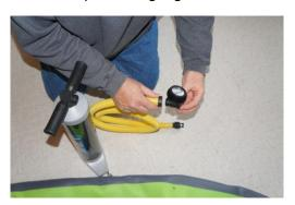
4. Attach other end of hose to the inflation/deflation valve on the rear of the board as shown below.
