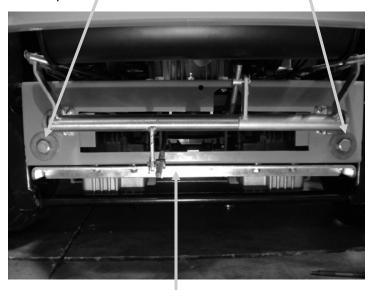
2. If necessary bump the bottom part of the mower with a tool lightly where the hydro systems are located to ensure the system is disengaged
