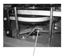
4. The brake pad material should be approximately 1/8-inch thick. Replace the brakes if the material is less than 1/16-inch thick.
