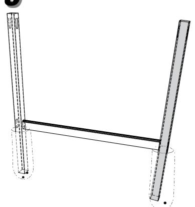
Next, attach U-Channels to boards (If applicable). If assembling Red Cedar panels, you must screw U-Channels to post first and then add boards.
