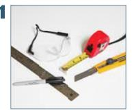
Tools Required: Straight edge, utility knife, tape measure and safety goggles
