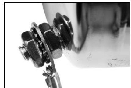
Step 16 - Install Nut on Stud against Washer & Tighten with 7/16" Wrench
