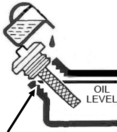
Figure 2 - Add Oil To TOP Of Threads
