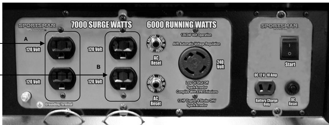
Figure 8 - Outlets Available on this Generator: 120V AC (4 each), 240/120 AC (one each) and 12V DC (one each). Output A Set of 2 Receptacles has max 20 Amps. Output B Set of 2 Receptacles has max 20 Amps. 240V Receptacle has max 30 Amps.
