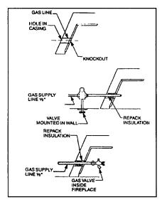
Figure 3 - Gas line installation Prefabricated fireplace
