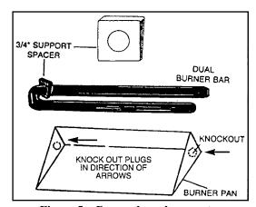
Figure 5 - Burner bar placement
