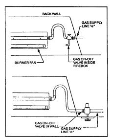
Figure 3 - Gas line installation Masonry fireplace
