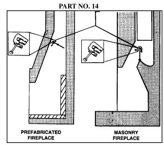
Figure 2. Damper stop clamp
