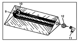
Figure 6 - Burner bar connection
