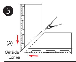
For outside corners (A) or inside corners (B), mitre cut both adjoining sections. Notch the front edge of one section to create an overlap.
