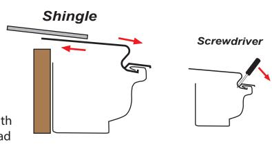
To overlap the gutter covers, cut a notch from the front edge. As you install each section simply overlap the end with the previous section.
