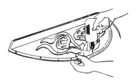
Mount clips to Window Well Cover using bolts and cap nuts provided. IMPORTANT! Put bolt through clip, cover and washer. Secure using cap nut provided (see below).
