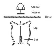
Snap Window Well Cover onto rim of window well. Adjust tension clips by loosening or tightening cap nuts. Your Window Well Covers are now easily removable for cleaning and ventilation.
