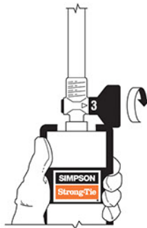
9. Turn the black valve to the #3 position and remove the black cap from the end of the nozzle. If performing gravity feed, the material is ready to dispense. If performing pressure injection, attach the E-Z-Click™ injection fitting to the end of the nozzle.
