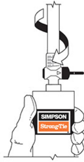
2. Screw the threaded portion of the nozzle into the cartridge.
