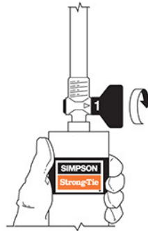
3. Turn the black valve so that the #1 on the valve aligns with the arrow on the neck of the nozzle.
