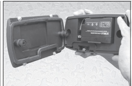
D. Reassemble Mounting Base and Electronics Console by Pushing the Two Pieces Together Firmly.
