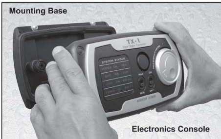
A. Separate Mounting Base From Electronics Console.
