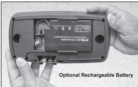
C. Install Optional Rechargeable Battery if Desired.
