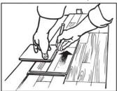
For the last row, install the long side tongue into the groove with the end joint aligned. Using a pull bar and hammer, work evenly along the length of the plank and lightly tap the joint closed.
