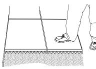
5 Step on blocks to dig block's teeth into the ground and position the blocks securely in place.
