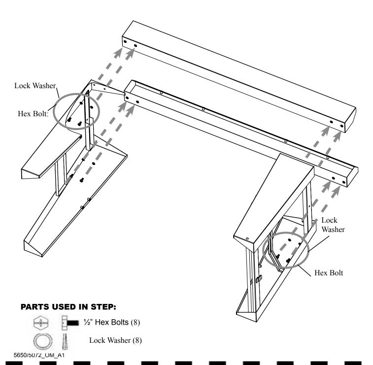
**Step 2** Attach FRONT & BACK CART BRACE to LEFT LEG WELDED ASSEMBLY and RIGHT LEG WELDED ASSEMBLY using four (8)  $\frac{1}{4}$ -20 x  $\frac{1}{2}$ " HEX BOLTS.
