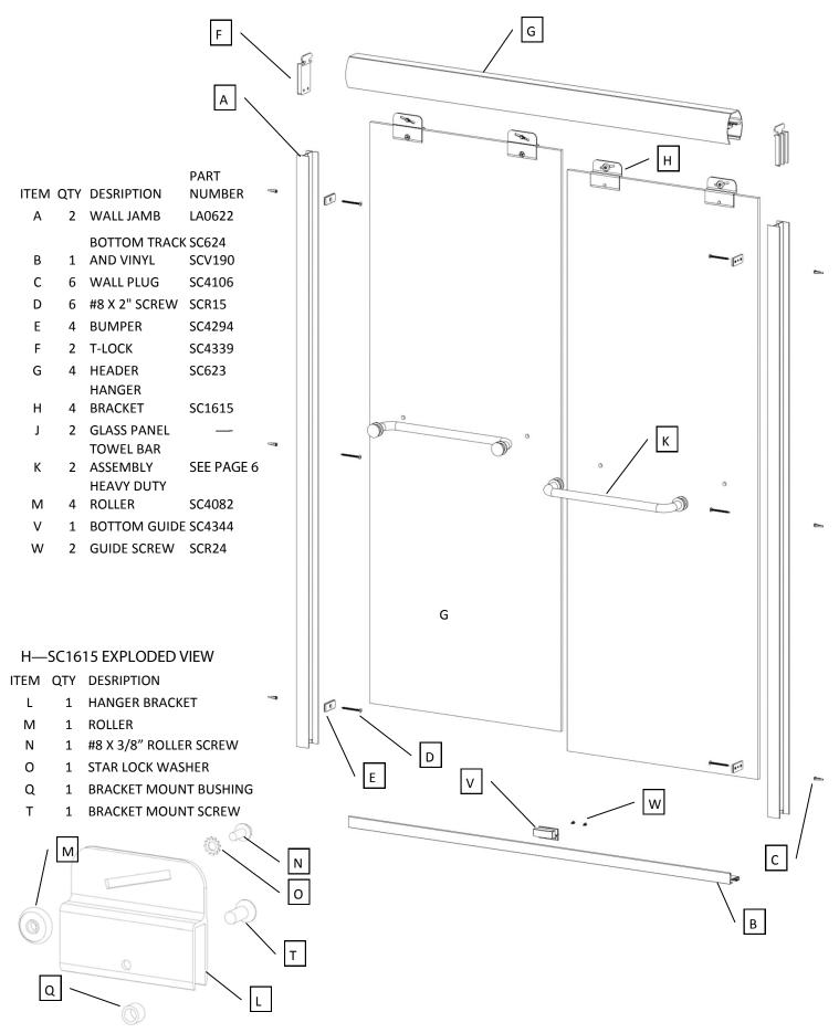
This framess bypass sliding enclosure is supplied with custom fit **Wall Jambs** [A]. The jambs are notched one end to fit over the bottom track.
