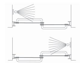
Measure the wall-to-wall opening along the center of the threshold at the bottom. Cut the **Bottom Track** (W/ Vinyl Silencer) [B] 1/16" short of that dimension.
