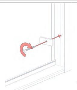
This enclosure is equipped with molded nylon **T-Locks** [**F**] for safety. When properly installed, the header is locked in the wall jambs and cannot be accidently removed.
