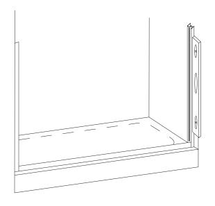
4 Before replacing the track, force a slight downward bow into it. This will ensure that the track fits tight to the threshold in the middle.
