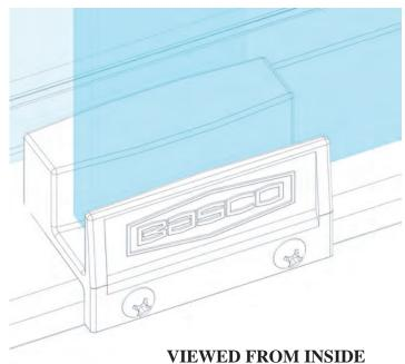
11 Neatly silicone each end of the tub track where it fits into the wall jambs as well as the seam between the wall and the wall jamb and the curb and threshold on the inside of the shower.
