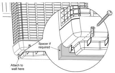
Note that if the cooler does not fit hard up against the outside wall (e.g. a protruding timber or brick window sill), utilise a spacer block of wood (not provided) which must be attached to the wall (the unit is then fixed to this wood).
