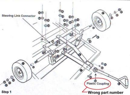
Turn the cart Bed(1) upside down. Use the cardboard from the carton to keep from scratching or damaging the finish.
