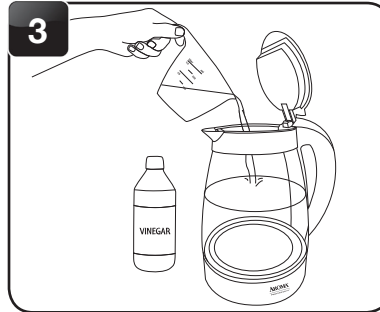
3 Add one cup of white vinegar to the water in the kettle.
