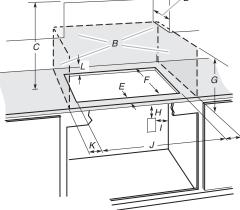
less than '/4" [0.6 cm] flame retardant millboard covered with not less than No. 28 MSG sheet steel, 0.015" [0.04 cm] stainless steel or 0.024" [0.06 cm] aluminum or 0.020" [0.05 cm] copper)
