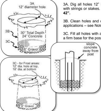
3A. Dig all holes 12" in diameter x 30" deep making sure not to interfere with strings or stakes. **Note: when using 9' posts, total depth should be 42"**.
