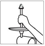
**3.** Slide the cover ring up to the ceiling and tighten the adjustment ring for a snug fit. (The cover ring should cover most existing recessed light rings.)
