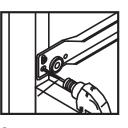
d make **2.** Drill 1/8" DIA. pilot hole in the second screw hole.
