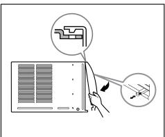
10. Put down inlet grille and take out the filter and secure it with 2 Type A screws through the front grille.
