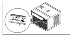
Attach the front grille to the cabinet by inserting the tabs the grille into the slots on the front the cabinet. Push the grille in until it snaps into place.
