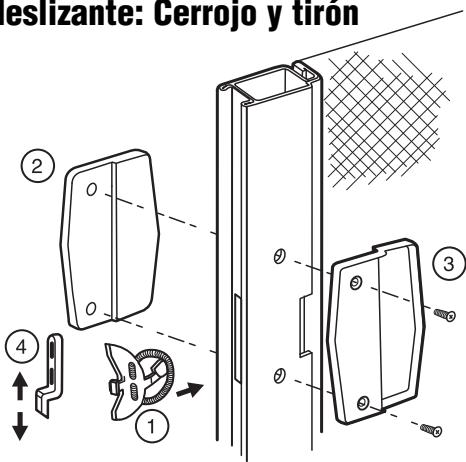
Remove old handles. Insert hook assembly (1) into latch opening and hold in position while installing outside handle (2). Be sure lever fits into latch slot in handle. Align inner handle (3) and install screws. Check for smooth operation and adjust strike (4) if necessary.
