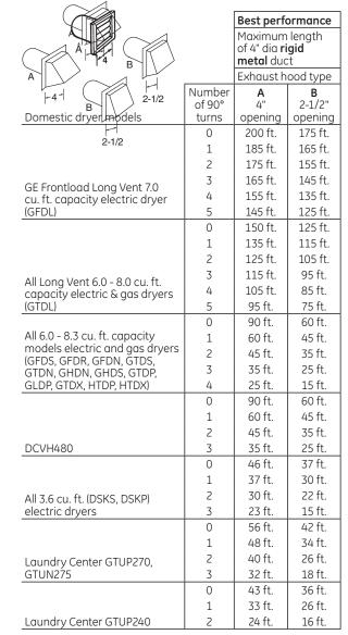
For every extra 90° elbow, reduce the allowable vent system length by 10 ft. Two 45° elbows will be treated like one 90° elbow.
