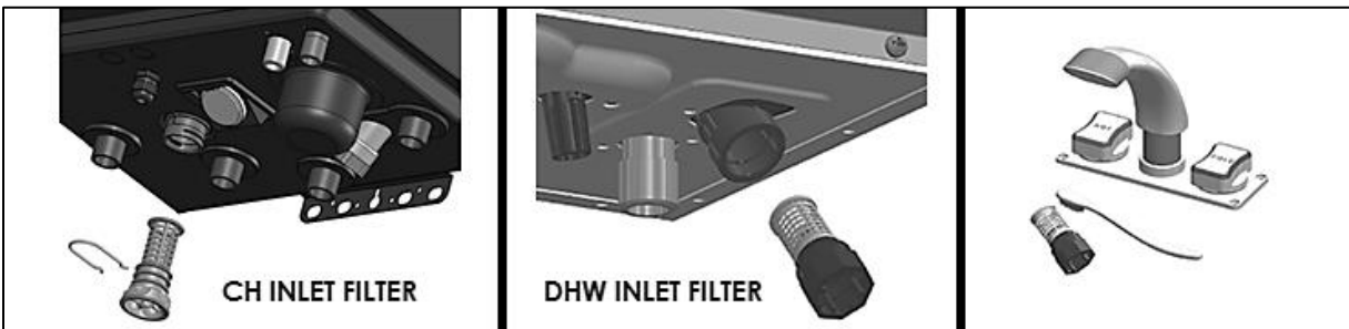
Figure 51 – Cleaning the Inlet Filter
