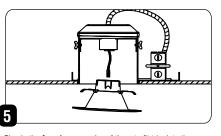
Plug in the **female connector** of the retrofit trim into the **male connector** of the socket adapter assembly.
