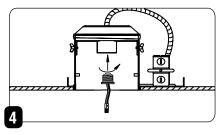
Thread the socket adapter into the socket
