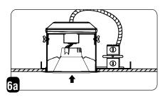
Push Downlight fixture into recessed housing.
