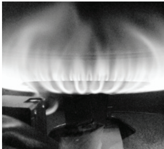
Proper burner flame pattern
