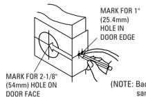
Start approximately 36" (914mm) from floor. Fold and apply template to edge of door and mark center of door edge as indicated on template. Mark center hole on door face through guide on template.
