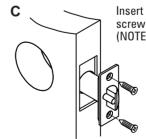
Insert latch and tighten screws.
